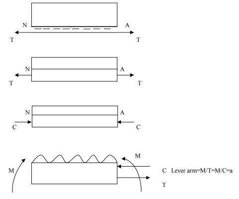
This concept is mostly used to determine the ultimate strength of pre stressed concrete member.
