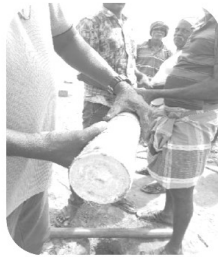
Figure 6. UDS sample collected at 7.0 m depth
