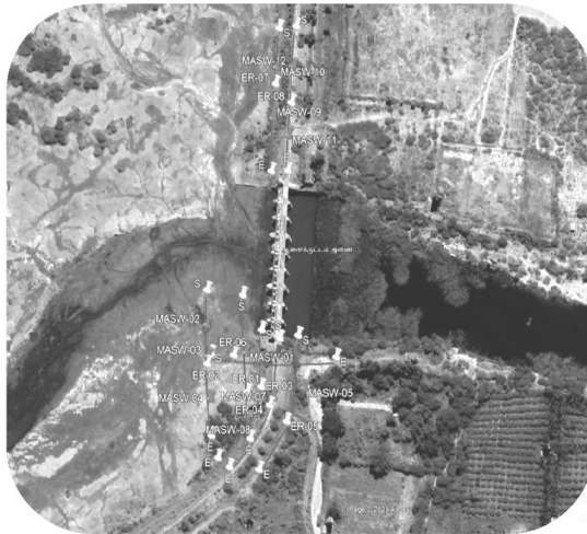
Figure 14. Locations of Geophysical resistivity survey and Multi-Channel Analysis of Surface wave
